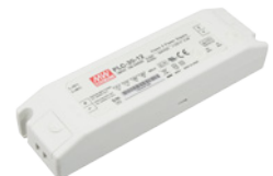
LED-DR30-12 12V DC Class 2 hardwire power supply 100-240V AC input, 1-30W 6-1/4"L x 1-1/4" H x 1-3/4"W c/UR/us Recognized for dry locations Can be used with AL-PWM-6A dimmer which consumes 3 watts
